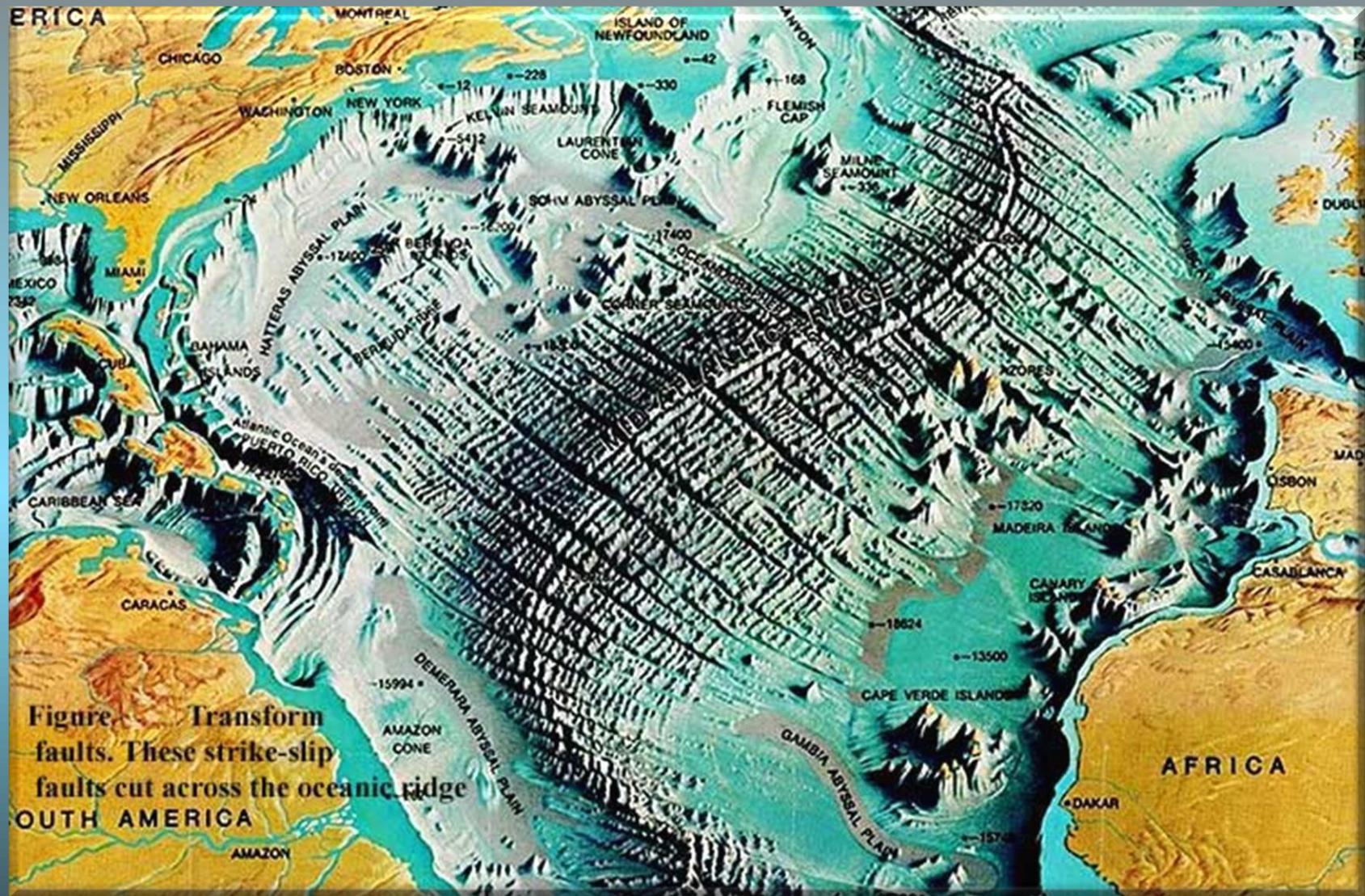
Figure 1. Transform faults. These strike-slip faults cut across the oceanic ridge.
